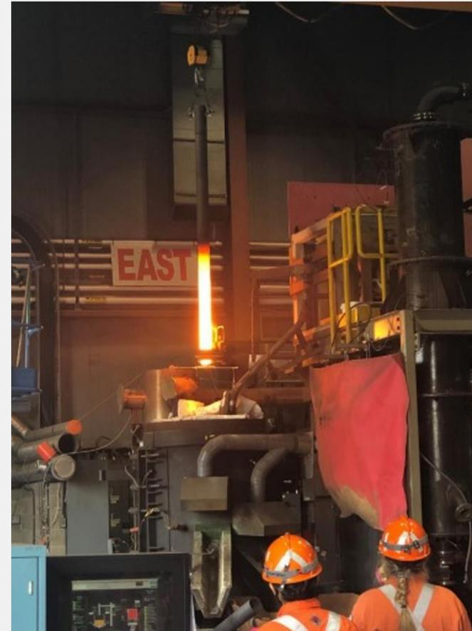
**Smelting** nodules in an Electric Arc Furnace at XPS facility in Canada. Electrode temperature 1450 degrees C. Smelting results in two products:
